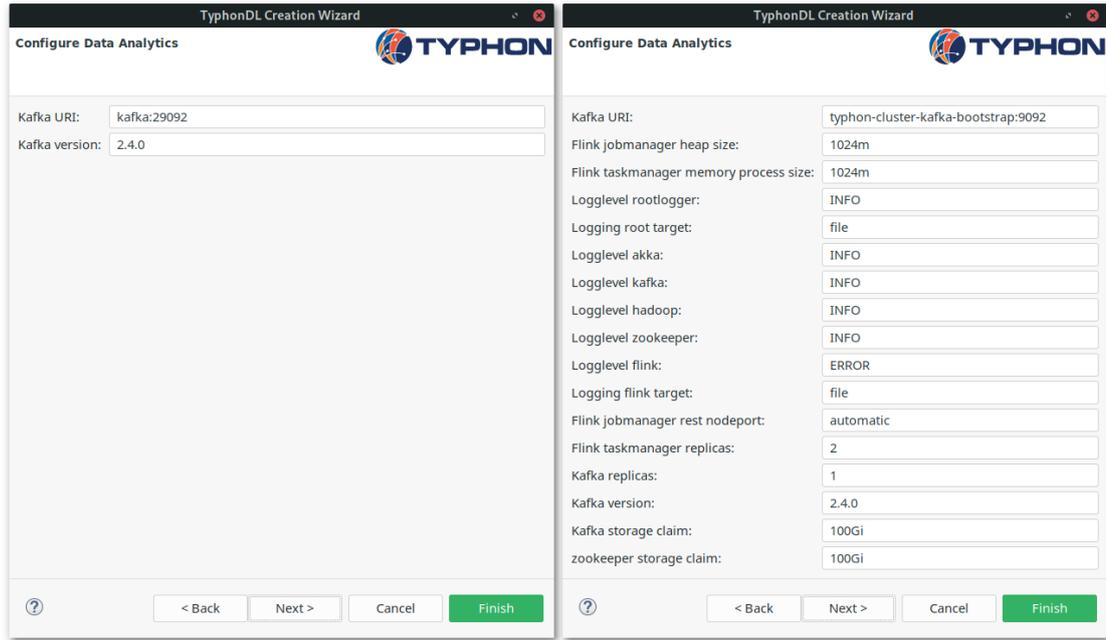
**Figure 3: TyphonDL Creation Wizard: Configuring the Analytics component Docker Compose vs. Kubernetes)**
