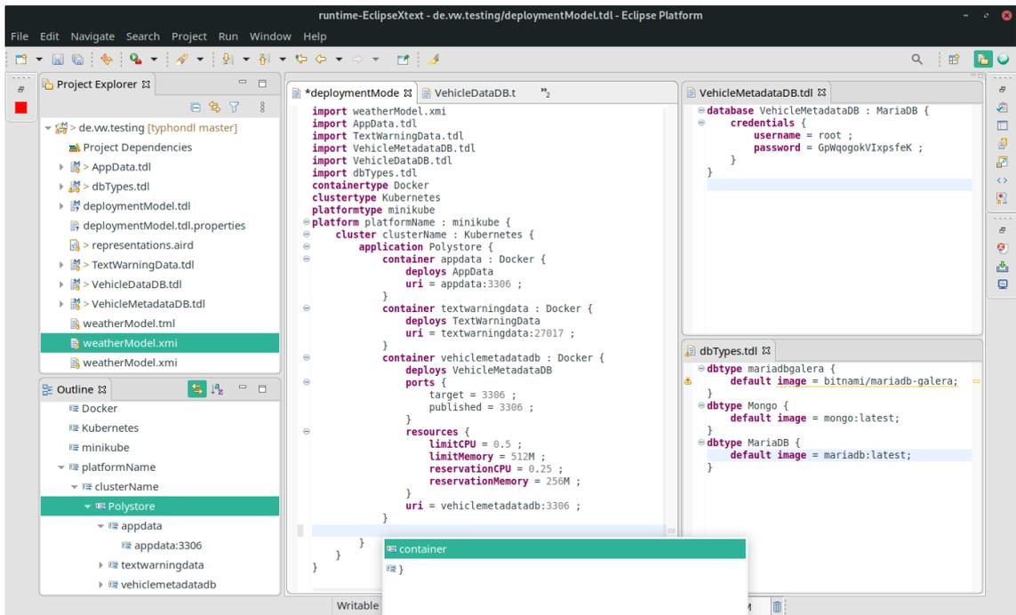
Figure 7: TyphonDL textual editor with syntax highlighting and auto completion
